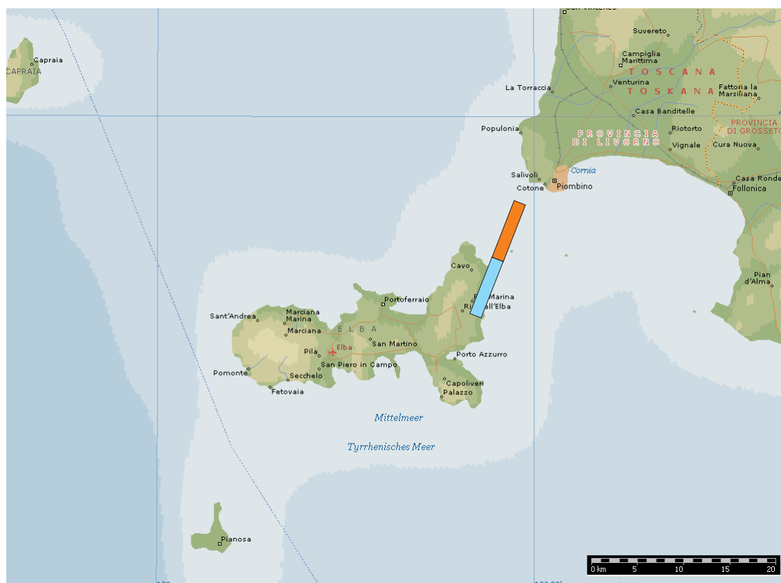
Figure 10.5: Geographical location of tropospheric \text{NO}_2 near the island of Elba (Italy). The colored bars indicate the AMAXDOAS footprint of a measurement. The orange bar represents the measurement at 9.099 UTC (9:05:56 UTC) and the blue bar represents the next measurement at 9.108 UTC (9:06:29 UTC).
