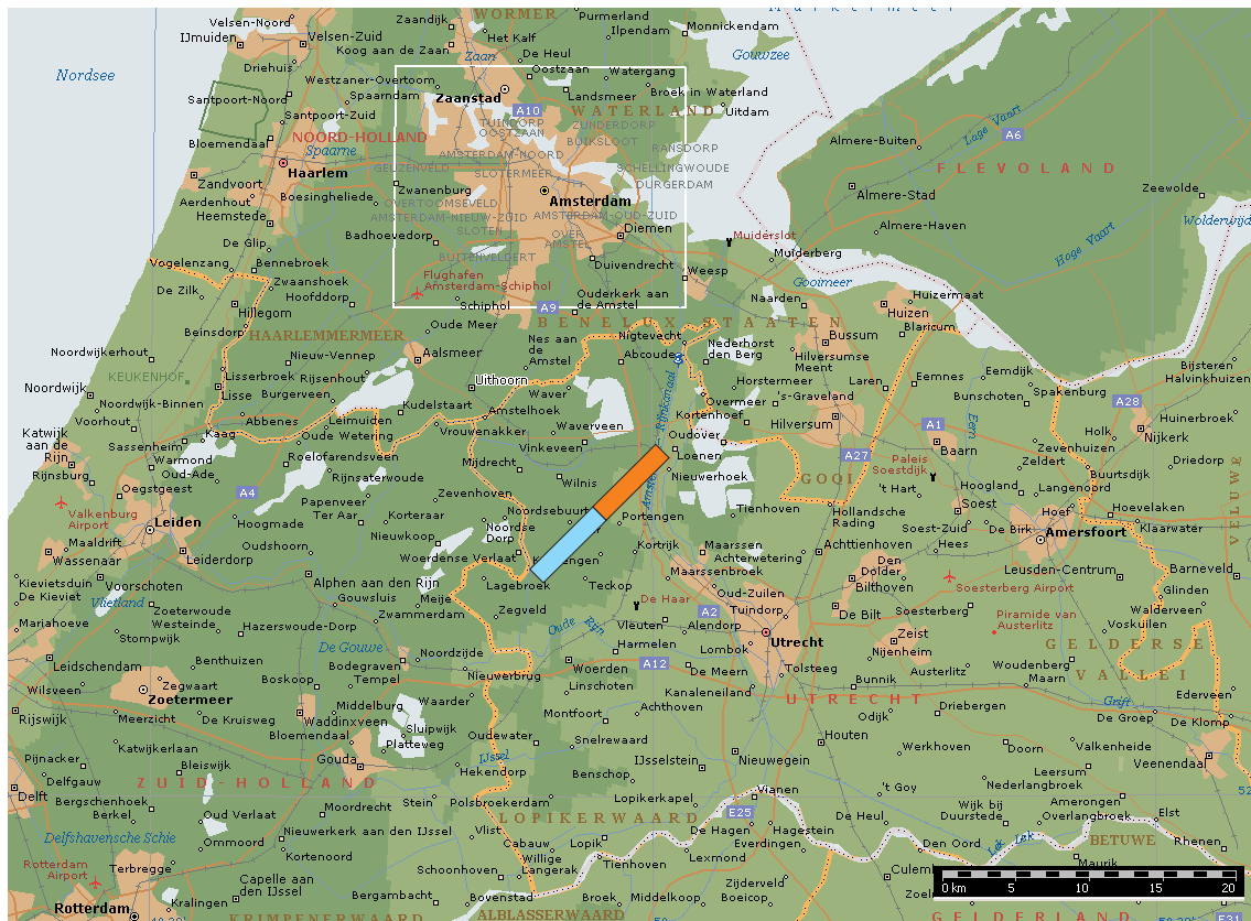
Figure 10.12: Geographical location of tropospheric \text{NO}_2 near Amsterdam (The Netherlands). The colored bars indicate the AMAXDOAS footprint of a measurement. The orange bar represents the measurement at 9.864 UTC (9:51:50 UTC) and the blue bar represents the next measurement at 9.873 UTC (9:52:23 UTC).
