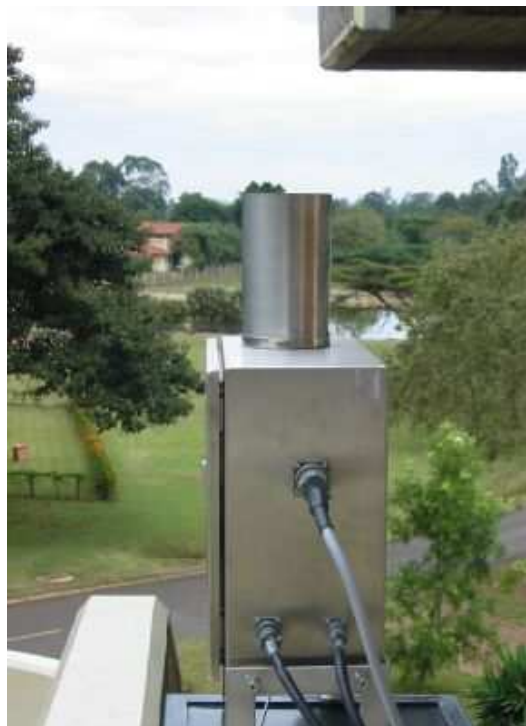
Figure 3.5: The telescope of the Nairobi MAX-DOAS instrument with off-axis directions facing ahead towards downtown. (University of Bremen, IUP)
