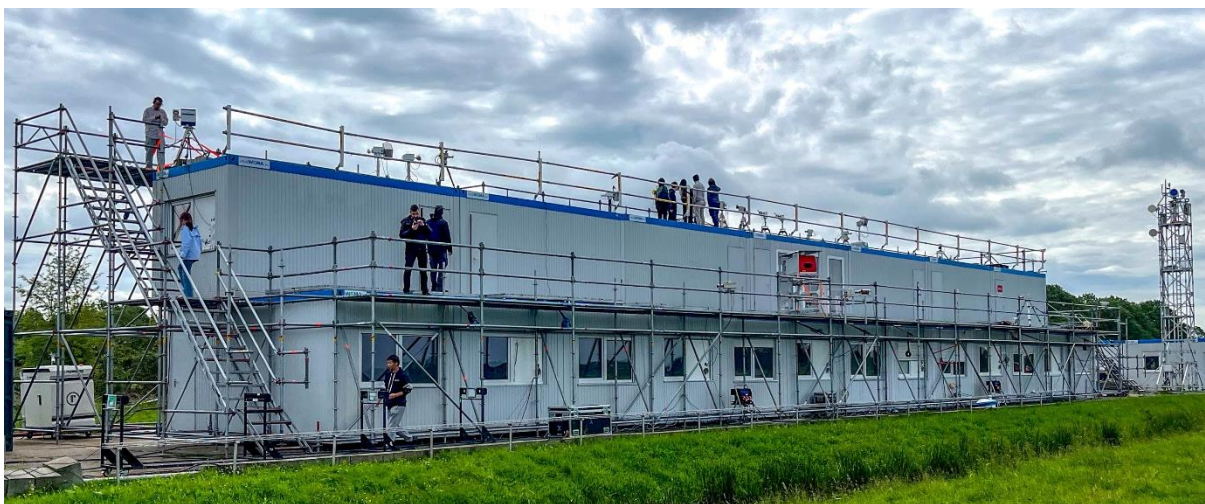
Fig. 8.2: Image showing CINDI-3 measurement site with instruments (outdoor parts) on the roof of the containers housing the instrument (indoor parts).
