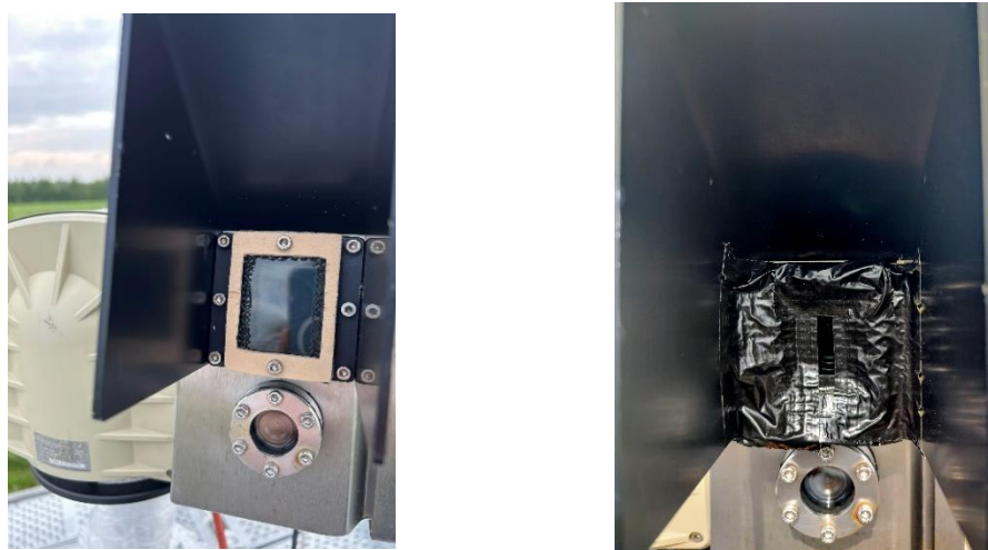
Fig. 5.1: (left) IMPACT telescope window as on May 30, (right) partial covering using black insulation tape installed.
