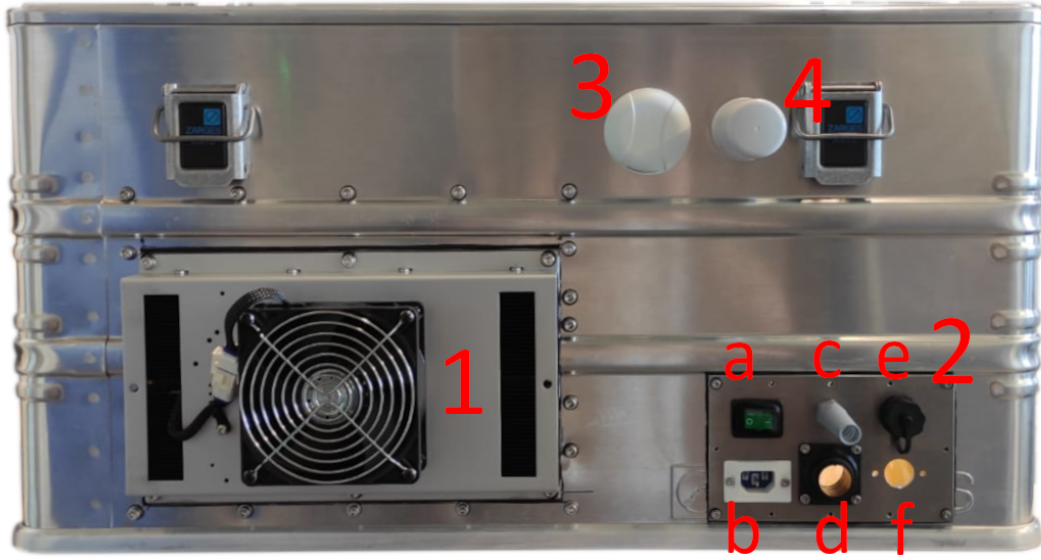
Figure 3.6: Modified Zarges Box with the components 1) TEM, 2) cable connector plate with a) power switch, b) power entry connector, c) cable gland for optical fiber, d) connector for pan-tilt head, e) RJ-45 jack, f) opening for HgCd lamp connector, 3) GNSS antenna, 4) LTE antenna
