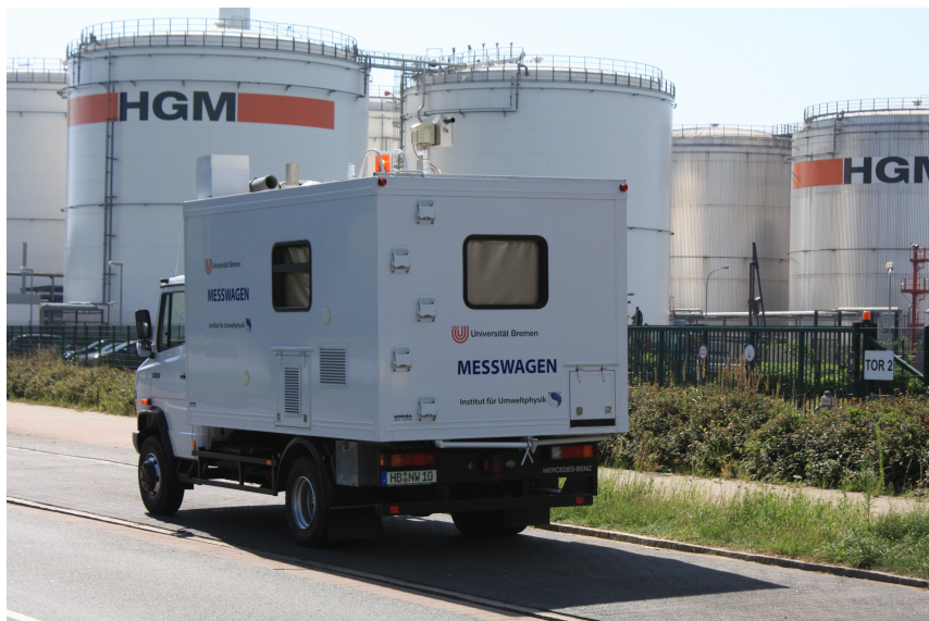
Figure 8.1: IUP-Bremen measurement car in the field performing MAX-DOAS measurements close to highway, industrial harbour and steel plants.
