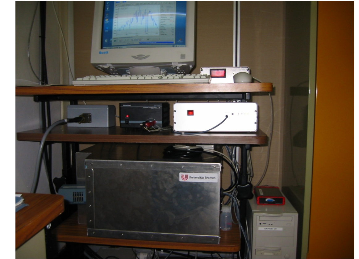
Figure 2: Inside equipment of the MAX-DOAS instrument with Spektrometer, CCD and PC
