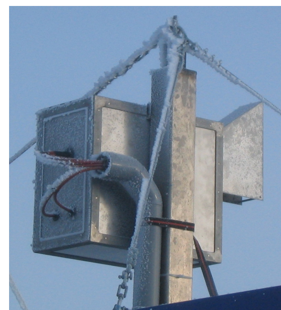
Figure 4: View of the DOAS telescope on top of the RAMAS container.
