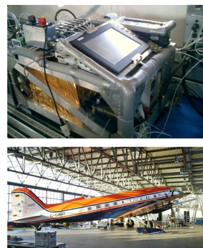
Photographs: (top) iDOAS installed in the Polar-5 aircraft (bottom) Polar-5 in the hangar at Bremerhaven regional airport
