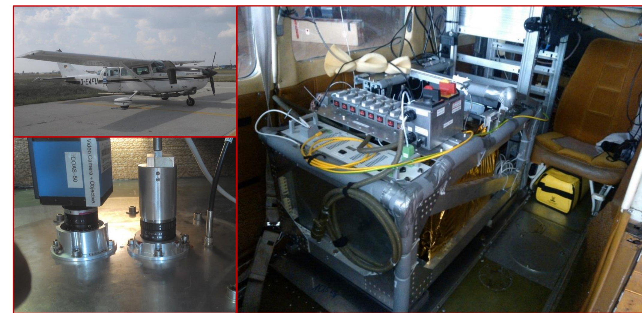
Fig. 1: Instrumental setup Scattered sunlight from below the aircraft is collected and fed into an imaging spectrometer via an sorted fiber bundle (35 individual fibers), retaining the spatial information.
