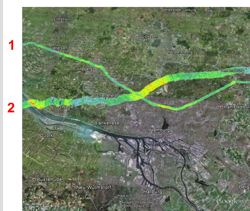
Fig. 7 (left): NO 2 observations during two overflights over the city of Hamburg (same colour scale as Figs. 4 & 9). The flight altitude determines the width of the swath.
