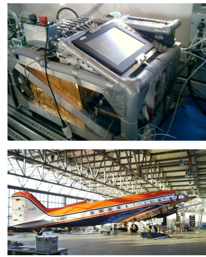
Photographs: (top) iDOAS installed in Polar-5 aircraft (bottom) Polar-5 in the hangar at Bremerhaven regional airport
