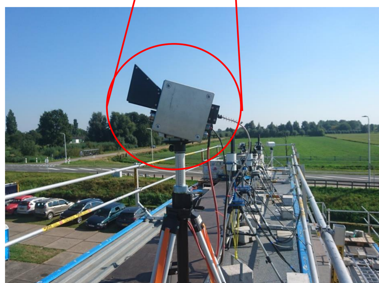
Fig 3: Telescope providing 50 elevations simultaneously, mounted on pan-tilt-head for azimuthal movement.
