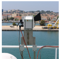
Figure 2: DOAS telescope installed on Kommandor Iona
