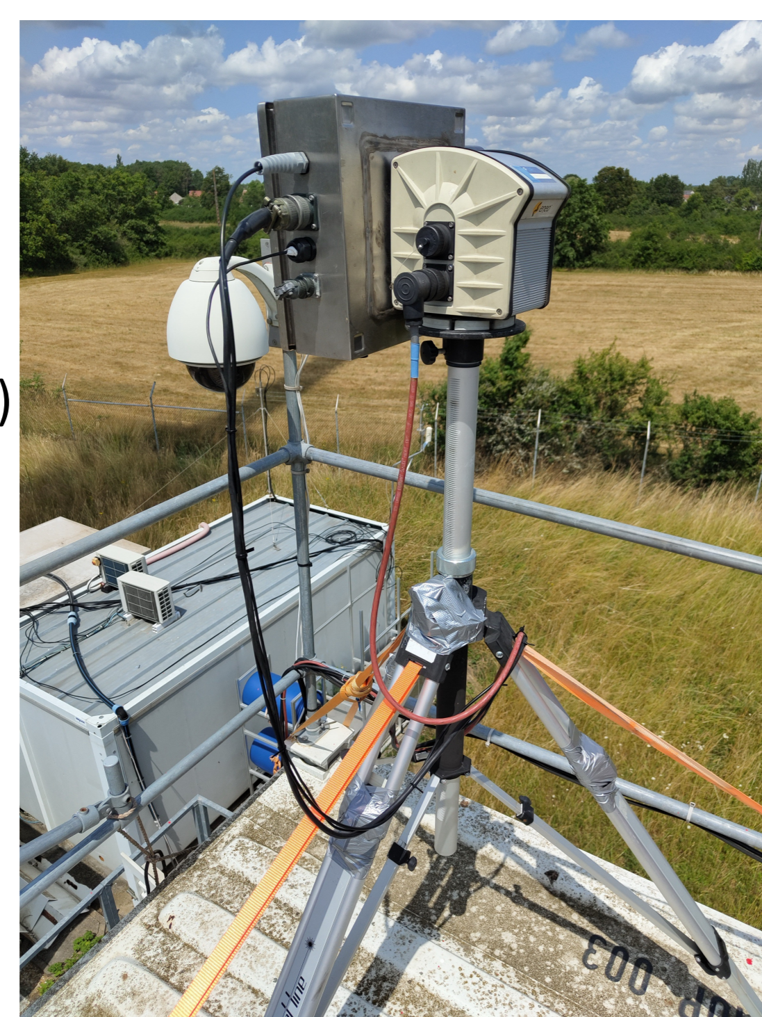
The backside of the telescope of the MAX-DOAS instrument on a tripod from Orléans.
