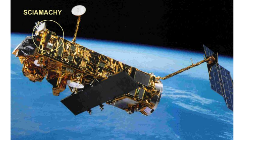
SCIAMACHY onboard ENVISAT, Monitoring the Changing Earth's Atmosphere, published by DLR, 2006. (ESA, artist's impression)
