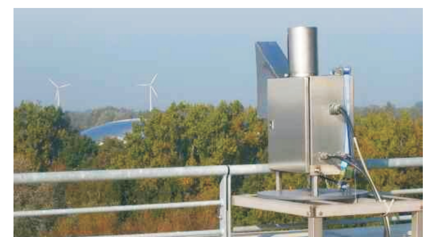
Figure 7: Photo of the MAX-DOAS telescope on top of the iup building in Bremen. The Bremen DOAS instrument provides a continuous time series of atmospheric trace gases like ozone and NO 2 , as well as BrO since 1993.
