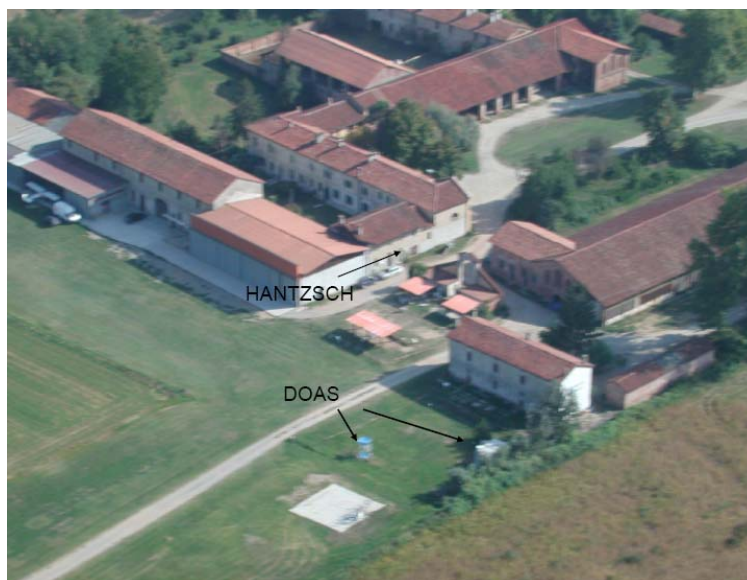
Fig. 6.1100.4: The farm buildings and hangars of Spessa in 2003. In the front are the DOAS container and the mirrors for four different viewing directions. The Hantzsch inlet was situated in 2.5 m above ground and 80 cm from the building. Sampling position from DNPH cartridges was on the southern side of the farm buildings in 2.5 m above ground on top of a container.
