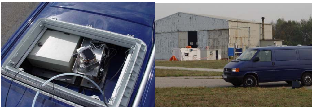
Figure 6.1300.4. 360^\circ rapid solar tracker connected to a 0.5\text{ cm}^{-1} resolution FTIR, operating at wavelength 2.5\text{--}14\ \mu\text{m} (left) and solar measurements at Bresso airport (right).
