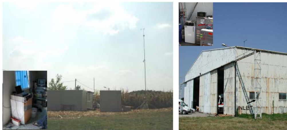
Fig. 6.1000.3: Instrument setup for Hantzsch in situ monitors at Alzate and Bresso. Three containers plus the mobile NILU DOAS were used for DOAS, Hantzsch in situ and VOC measurements. Air sampling for Hantzsch and DNPH cartridges were done half a meter above the roof of the left container. In Bresso the instrument was placed in the old hangar, the inlet was about 6 m from the building.
