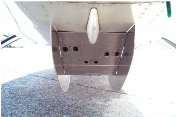
Figure 6.2200.1: Upper photo: The Partenavia aircraft and the two telescope boxes fixed above and below the aircraft, respectively, as used during the first campaign. Lower photo. Improved telescope box as used during the second campaign
